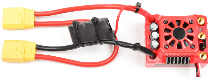
Secure the capacitor wires to the ESC wires with 2 tie-raps. Then solder the wires together.
