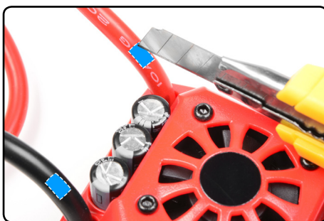
Using the cutter, carefully cut a window in the ESC cable insulation to reveal the strands. Be careful not to cut the strands !
