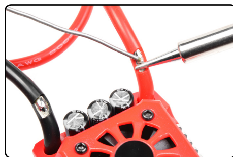
Using the soldering iron, preheat the strands for a few seconds and then apply the solder. Only the surface strands must be tinned.
