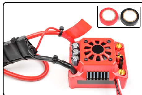
Use electrical insulating tape to protect against oxidation.
